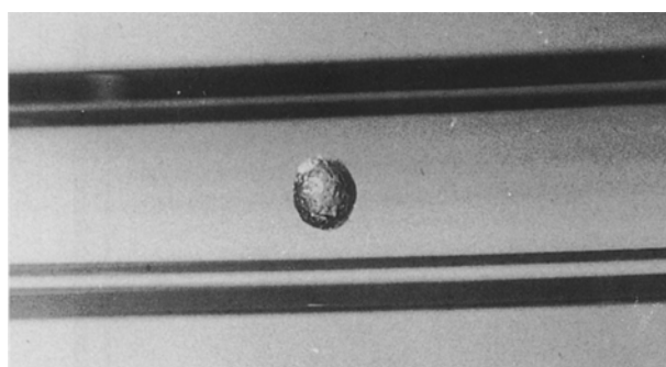
Figure 8 Final appearance of a shrinkage defect in Range II of the cure temperatures.
